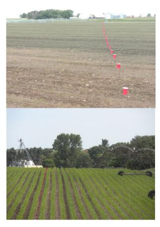
Pictured above, irrigation "catch cans" are used to test whether nozzles are functioning properly.
