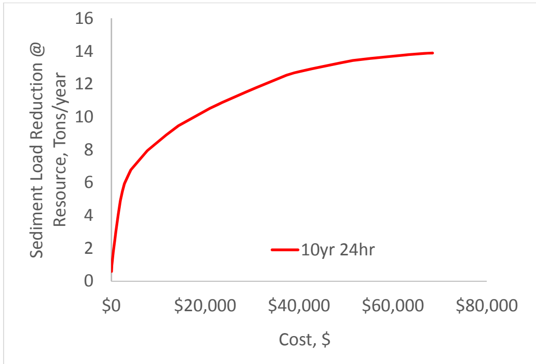
Figure 8. Single treatment efficiency frontier for filtration practices. Frontier indicates the maximum reduction in sediment delivered to the main channel of the Sand Hill River relative to the implementation cost.
