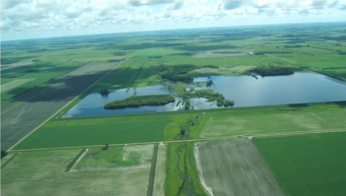
Figure 9. Brandt impoundment, Red Lake Watershed District located on a small altered natural watercourse. Designed to detain 3,912 ac-feet of runoff.
