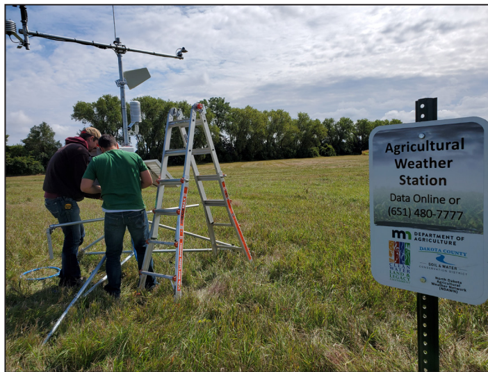
The Dakota County SWCD established a weather station about a mile south of Hastings to provide data for an online irrigation scheduling tool. Photo Credit: Dakota County SWCD
