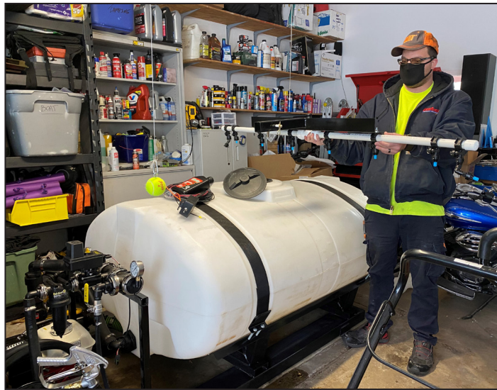
Cost-share funding from Scott WMO helped the city of Shakopee purchase a brine maker, shown above. Using liquid brine can make application more precise and efficient than using traditional de-icing salt. Photo Credit: City of Shakopee
