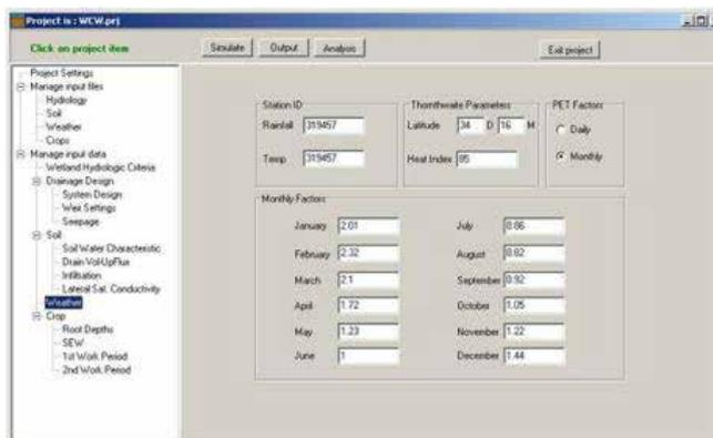
**Figure 19–78** DRAINMOD screen showing inputs for wetland analysis
