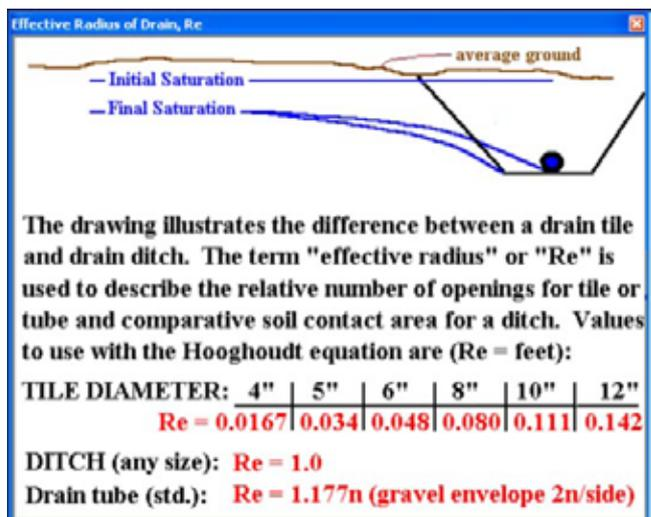
**Figure 19–74** Output from the Skaggs method
