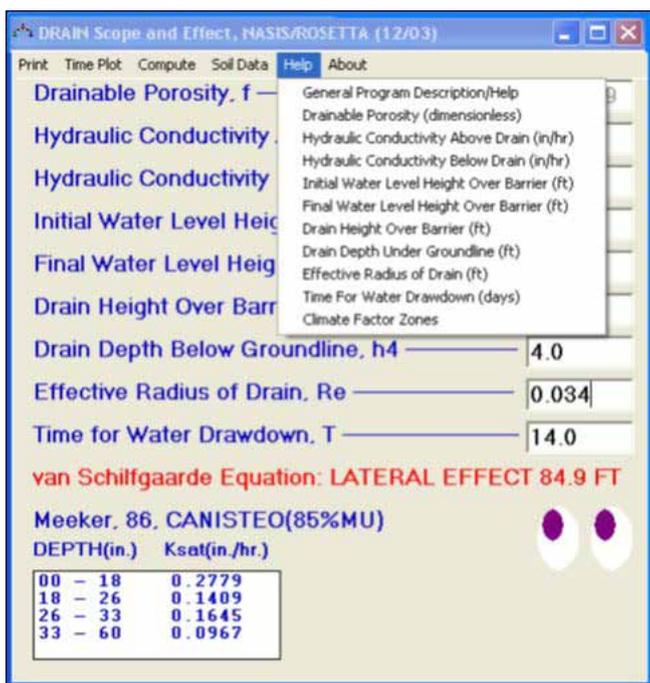
Figure 19–73 Help screen, drain effective radius, feet
