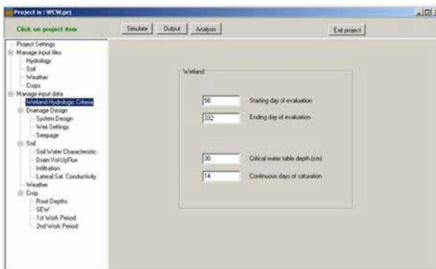
**Figure 19–80** Schematic view of DRAINMOD parameters
