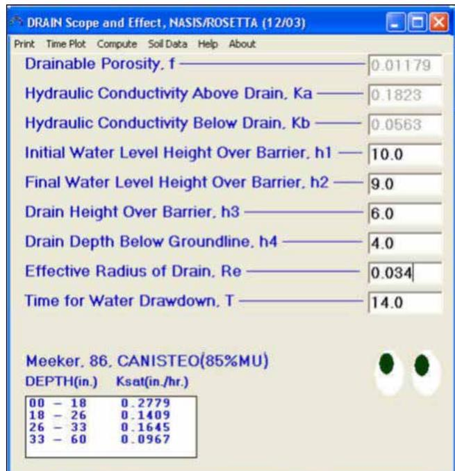
**Figure 19-71** Selection of lateral effect method screen
