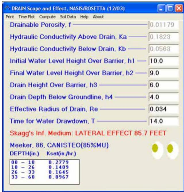
**Figure 19–75** Output from the Van Schilfgaard equation
