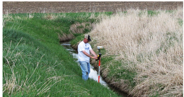
Figure 3.61 Surveying a Ditch Cross Section
