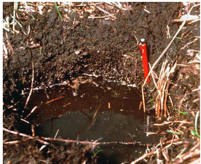
Figure 3.28 Measuring Water Levels in Test Pit
