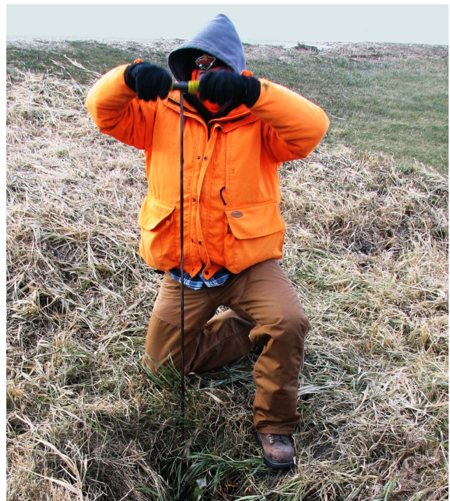
Figure 3.37 Probing for Drainage Tile
