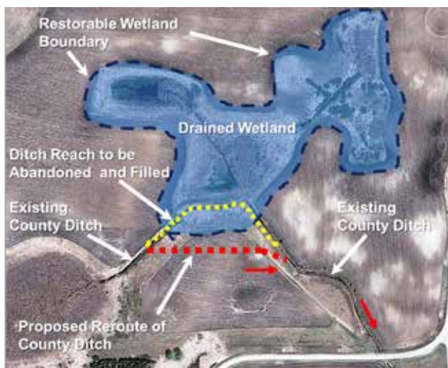
Figure 4.9.7 Typical Rerouted County Ditch System
