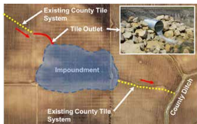
Figure 4.9.6 Wetland Restored Within County Tile System
